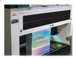
Enercon's leading atmospheric plasma treatment technology cleans, etches and functionalizes surfaces that would be otherwise unresponsive.
